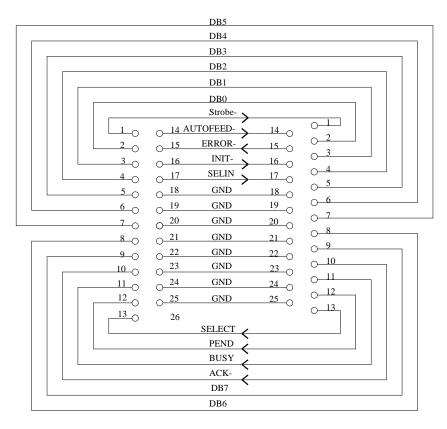
PCB Connector Female DB25 Connector Female
